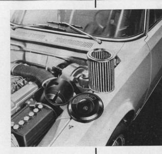
The fuel supply is effected by a mechanical pump located on the right-hand side of the engine and actuated by the distributor drive shaft. The fuel sucked by the fuel pump reaches the carburettor through a bowl filter on the right-hand side of the engine compartment.
